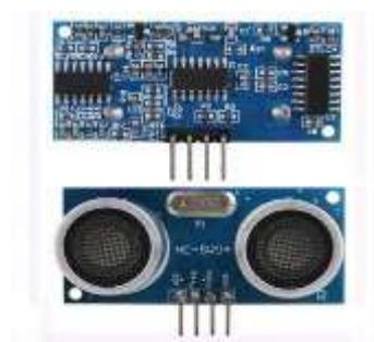
**Gambar 2.** Sensor Ultrasonic HC SR-04
